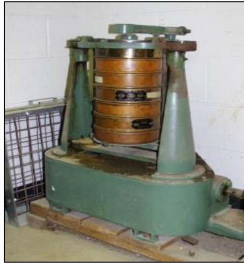
Figure 7. Set of sieves in a sieve shaker
